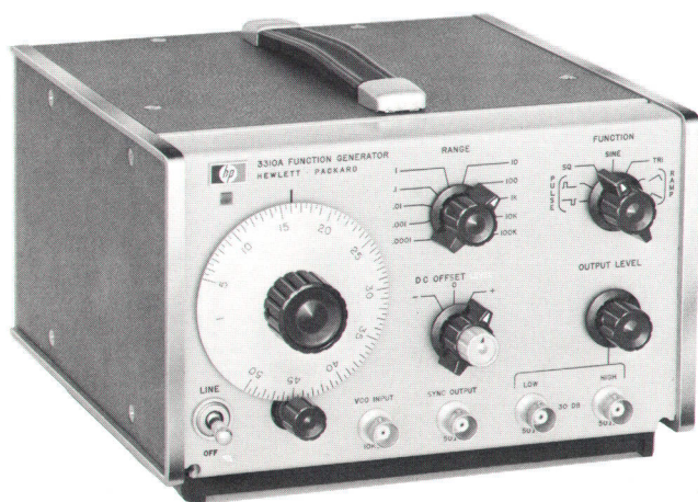
Fig. 1. This new HP Model 3310A Function Generator has a frequency range from 0.0005 Hz to 5 MHz and generates sine, square, and triangular waves as well as pulses and ramps.
